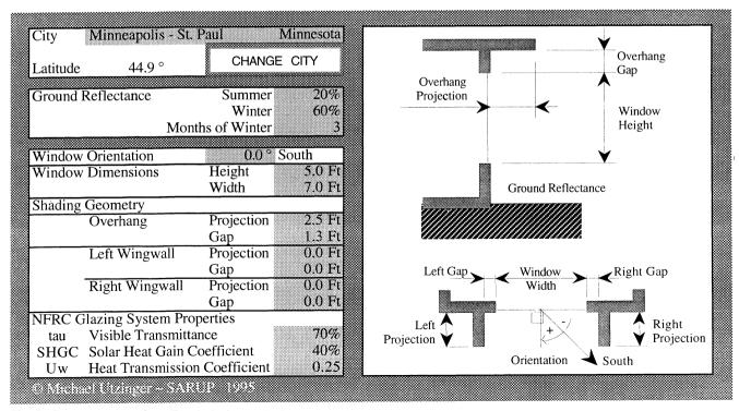
Fig. 7. Data entry page from Excel glazing analysis program *Glazing.xlw*.
