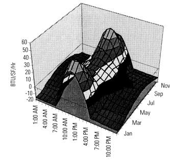
Figure 8: Average hourly heat flow across glazing for the year, an output graph from *Glazing.xlw*.
