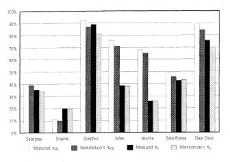
Fig. 2. Comparison of measured transmittance (visible and solar) with manufacturer's data for a variety of glass types. The manufacturer's data was drawn from the **WINDOW 4.1** database.
