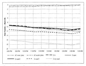
Figure 6: Heat flow across the glazing estimated from measured surface and air temperatures.
